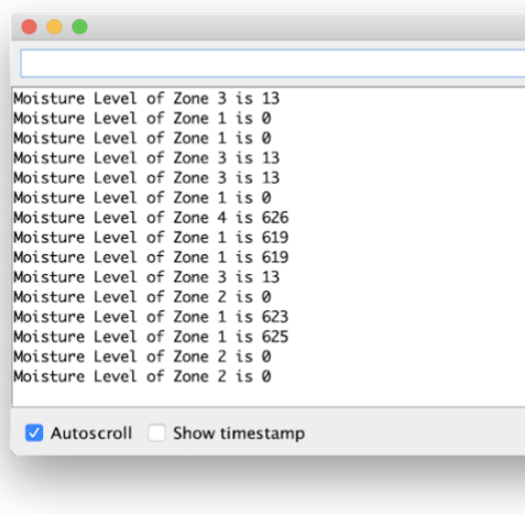
Figure 8: Main microcontroller receiving soil moisture levels from four zones.
